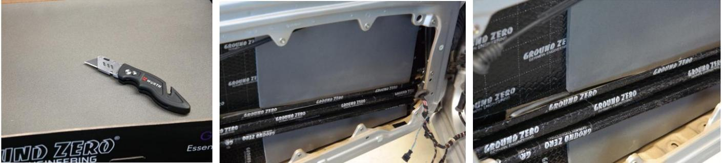
Step 7: Clean the surface of the back side of the door trim from grease and grime
