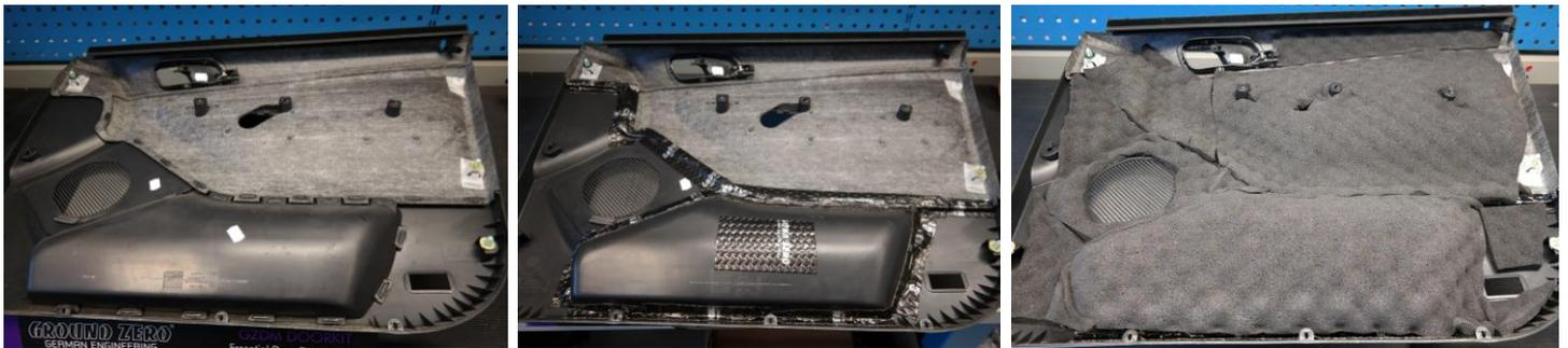
Step 10: Re-assemble the door trim and check the functions of the power window and switches
